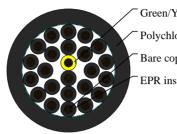
Green/Yellow wire Polychloroprene rubber outer jacket Bare copper conductor EPR insulation
